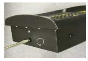
Step 2: If terminal has nylon waterproof screws on its sides, remove them (4 places)
