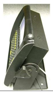
Finished: swivel terminal to most comfortable viewing angle
